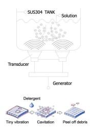
Ultrasonic cleaning is based on the cavitation effect caused by high frequency ultrasonic wave vibration signal in the fluid. Microscopic bubbles are formed, and then implode violently causing the cavitation which create an intense scrubbing action on the surface of the item being cleaned. The bubbles are small enough to penetrate microscopic crevices, cleaning them thoroughly and consistently.
